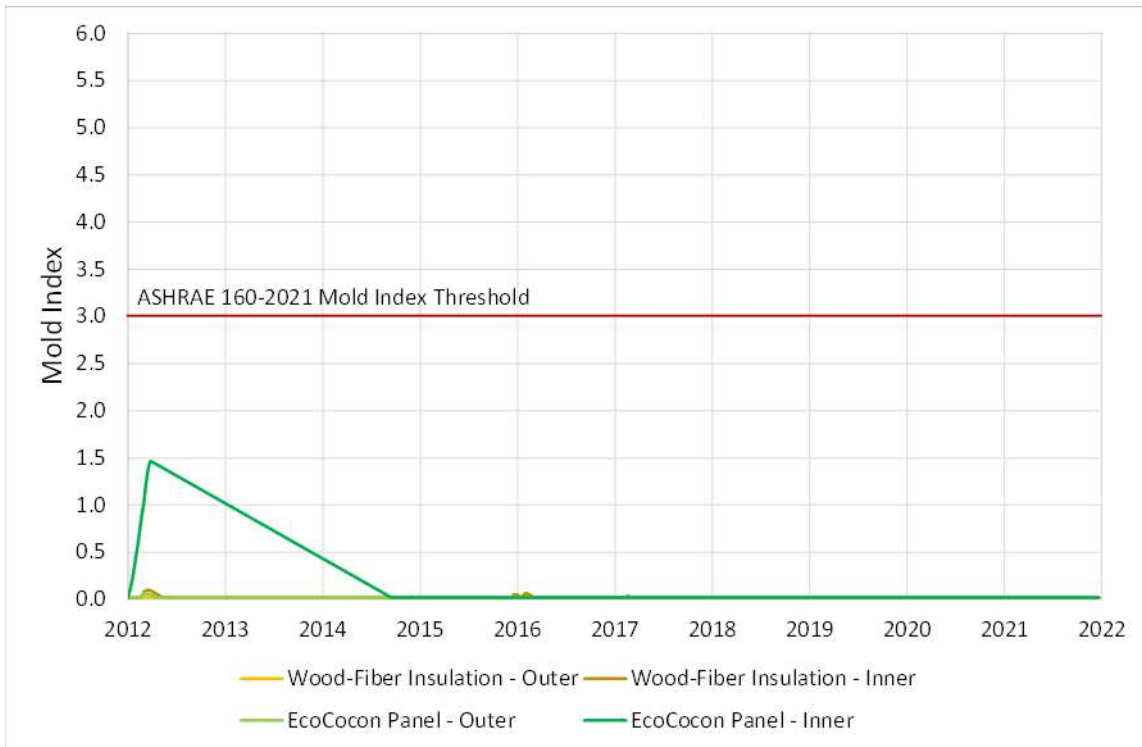
Figure 4.12 - Mold index graph: north oriented, 1% rain leak.
