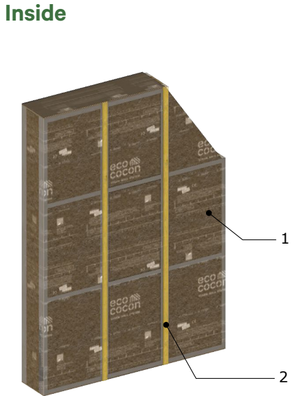
Membrane + thin plywood strips
