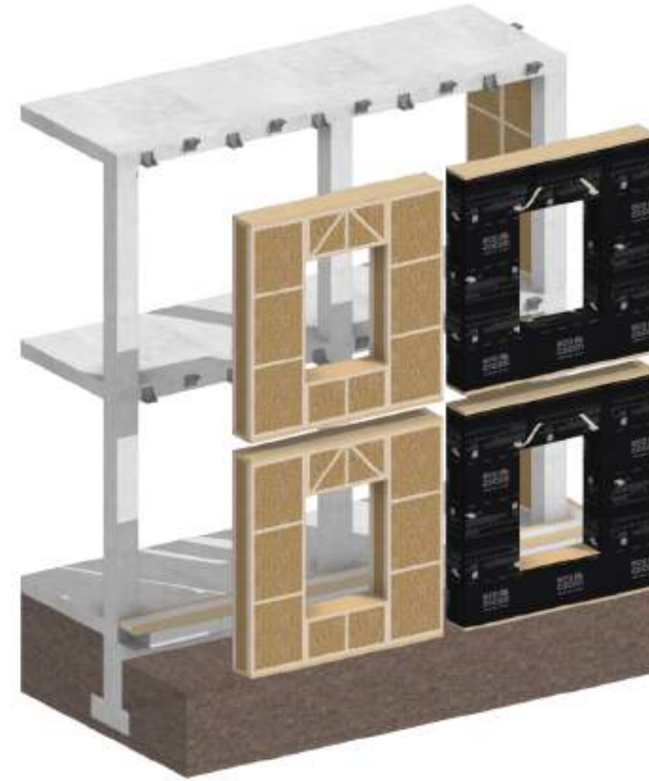
EcoCocon infill panels between concrete frame.
