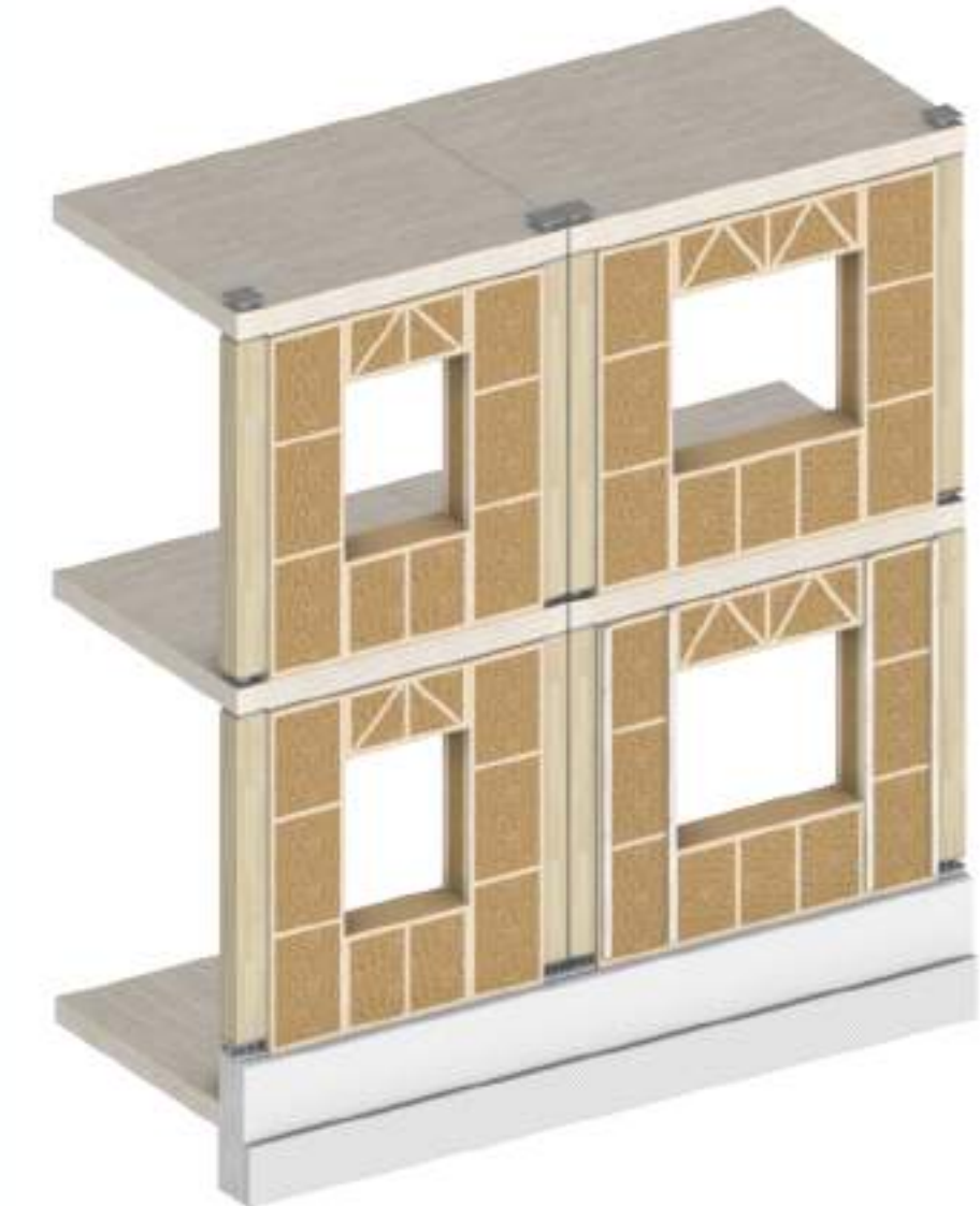
EcoCocon infill panels between timber frame.
