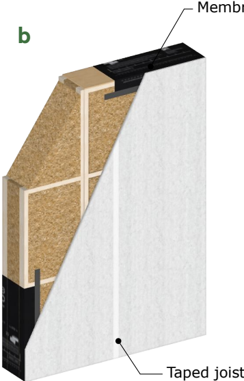
Protective board with taped joints
