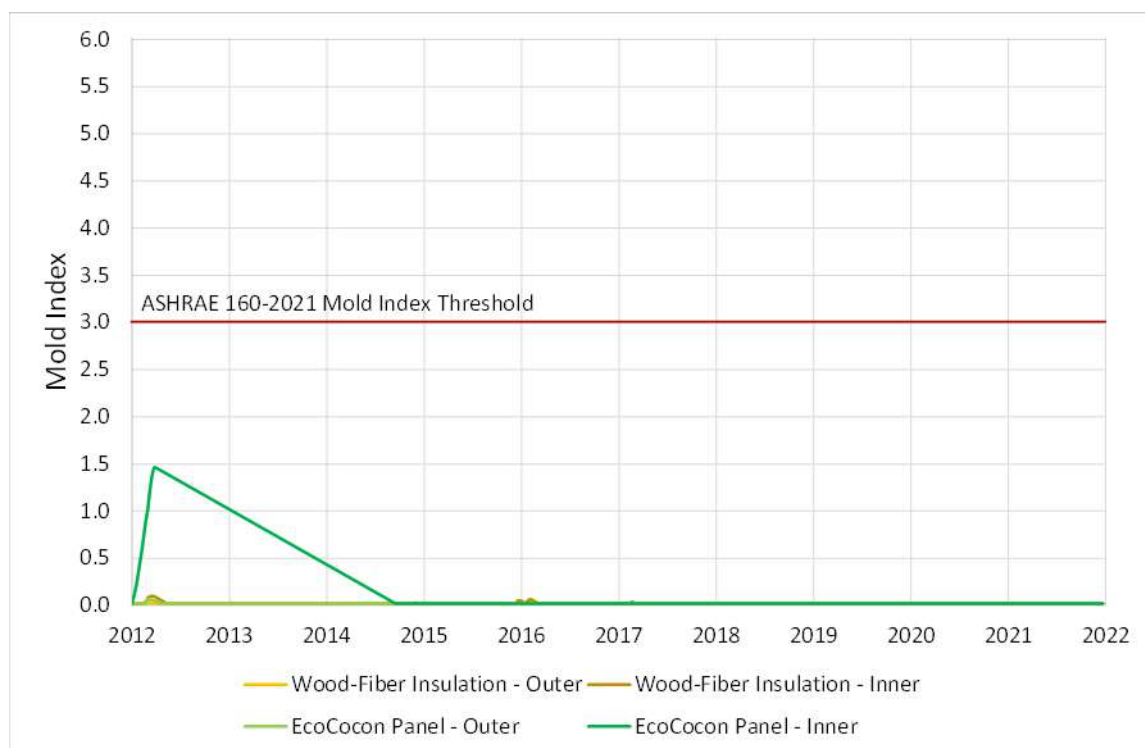
Figure 4.12 - Mold index graph: north oriented, 1% rain leak.
