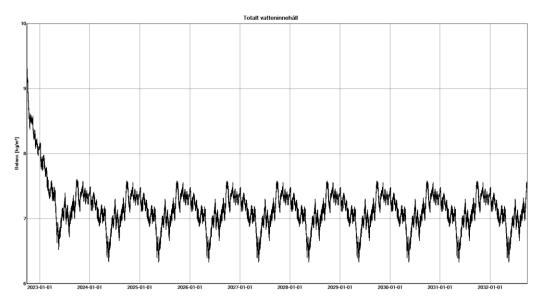
Even with high built-in moisture content (assumed at 80%), the entire wall structure dries out quite quickly. A simulation over 10 years shows that there is no accumulation of moisture over the long term. No risk of damage to the building fabric, or mould, can be expected if the work is carried out correctly. As the building consists of prefabricated modules, the risk of internal moisture or leakage is even lower.
