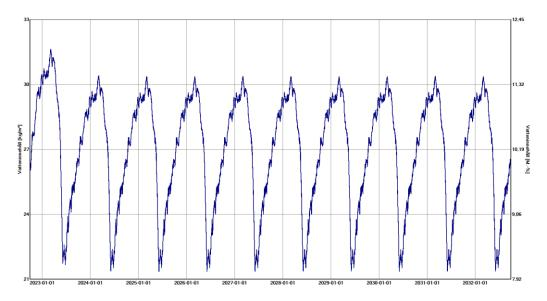
The wood fibreboard has the chance to dry out and the moisture content is always below 12 M.-% which is far below the critical limit.
