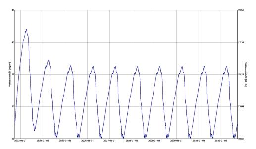
The wood fibreboard has the chance to dry out and the moisture content is always below 16 M.-%, which is below the critical limit.
