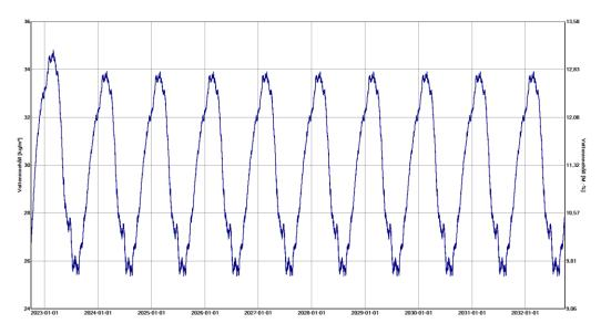
The wood fibreboard has the chance to dry out and the relative humidity is constantly below 13 M.-% and thus below the critical limit.
