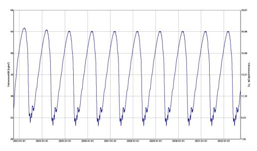
The wood fibreboard has the chance to dry out and the water content is always below the 18 M.-% which is considered the critical limit.
