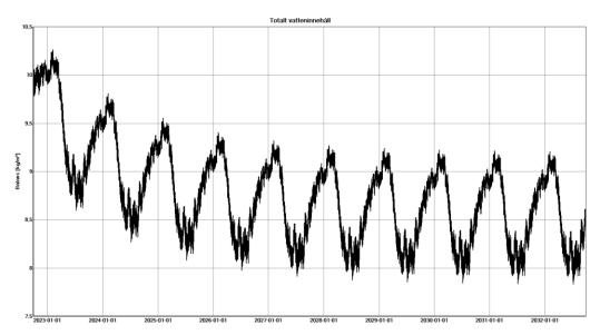
The simulation over 10 years shows that there is no accumulation of moisture over the long term, but it takes a few seasons to release the (unusually high assumed) built-in moisture. No risk of damage to the building fabric, or mould, can be expected if the work is carried out correctly.
