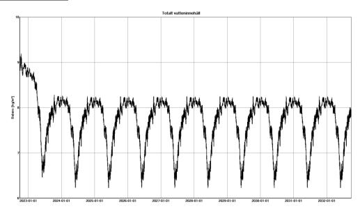
Even with a high built-in moisture content (80%), the entire wall structure dries out quite quickly. A simulation over 10 years shows that there is no accumulation of moisture over the long term. No risk of damage to the building fabric, or mould, can be expected if the work is carried out correctly. As the building consists of prefabricated modules, the risk of internal moisture or leakage is even lower.
