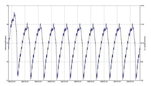
The wood fibreboard has the chance to dry out and the moisture content is always below 12 M.-% which is far below the critical limit.
