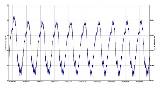
The asphalt fibreboard has the chance to dry out and the relative humidity is constantly below 16 M.-% and thus below the critical limit.
