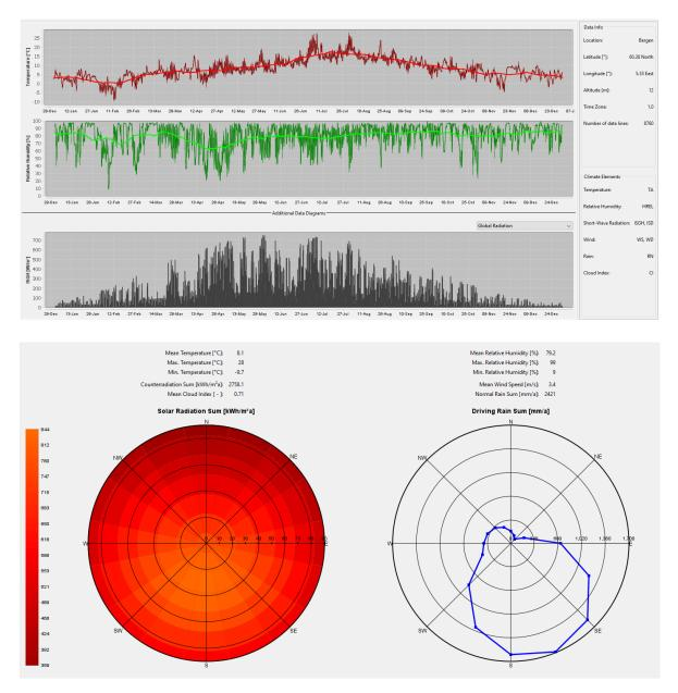
The direction with the most driving rain is south-southeast. There is a lot of solar radiation, with higher drying capacity than that towards most other orientations. Therefore, the southeast orientation is used for analyses of plastered walls, with still a lot of driving rain but slightly less drying capacity. For ventilated facades, the north orientation is always the decisive one.
