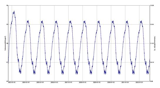
The wood fibreboard has the chance to dry out and the water content is then constantly below 13 M.-% and thus below the critical limit.
