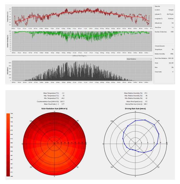
The direction with the most driving rain is northeast. There is also relatively little solar radiation, with lower drying capacity than that found, for example, towards the south. Therefore, this orientation is used for analyses of plastered walls. For ventilated facades, straight north is always the decisive orientation.
