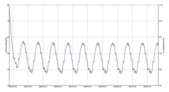
A low moisture level is reached after only a few months. Even with the intentionally high value at the beginning, the water content drops quickly and stays below 9 M.-%.
