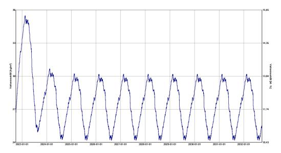
The wood fibreboard has the chance to dry out and the water content is always below 14 M.-% which is far below the critical limit.
