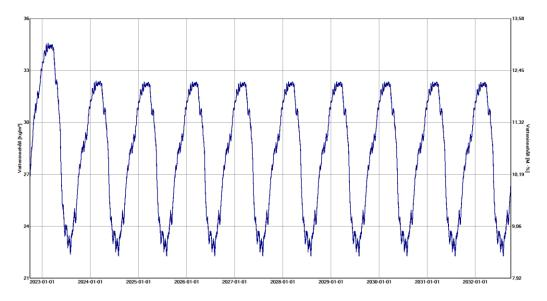
The wood fibreboard has the chance to dry out and the moisture content is always below 13 M.-% and thus far below the critical limit.
