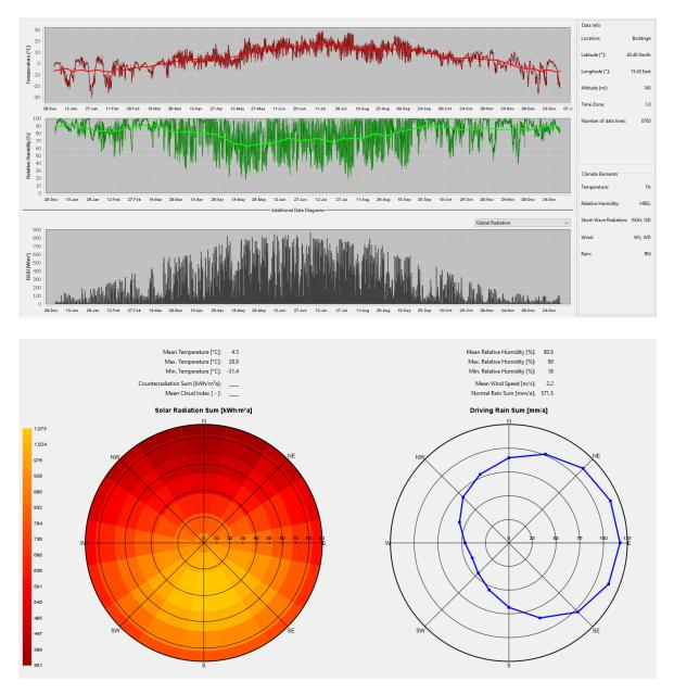
The direction with the most driving rain is east. There is also only moderate solar radiation, with lower drying capacity than that to the south. For analyses of plastered walls, the northeast orientation is used, as there is still a lot of driving rain there and also less drying from solar radiation. For ventilated facades, northward is always the decisive orientation.
