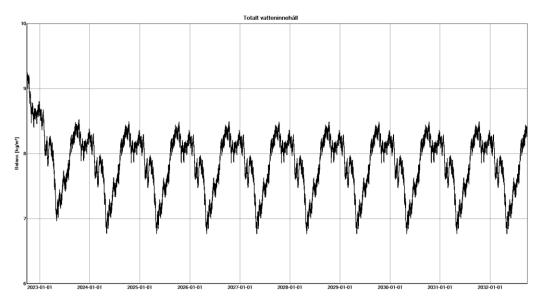
Even with a high built-in moisture content at the beginning, the entire wall structure dries out quite quickly. A simulation over 10 years shows that there is no accumulation of moisture over the long term. No risk of damage to the building fabric, or mould, can be expected if the work is carried out correctly. As the building consists of prefabricated modules, the risk of internal moisture or leakage is even lower.
