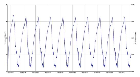
The wood fibreboard has the chance to dry out and the water content is always below the 18 M.-% which is considered the critical limit.
