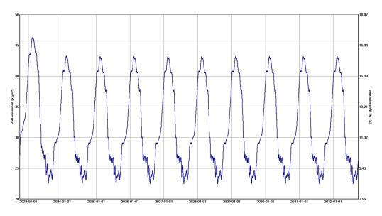
The wood fibreboard has the chance to dry out and the moisture content is always below 17 M.-% and thus below the critical limit.
