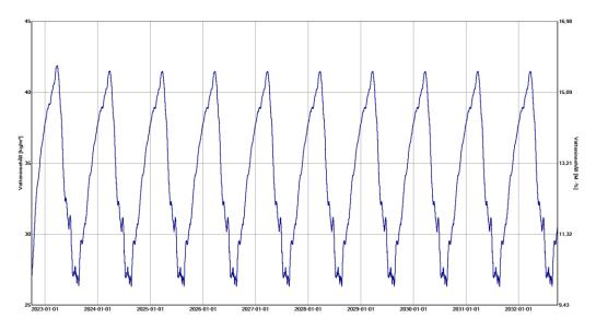
The wood fibreboard has the chance to dry out and the water content is always below the 18 M.-% which is considered to be the critical limit.
