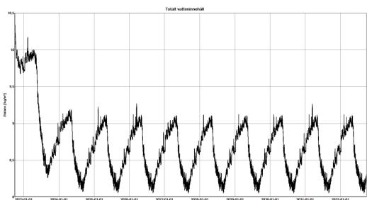
Even with high built-in moisture content, the entire wall structure dries out quite quickly. A simulation over 10 years shows that there is no accumulation of moisture over the long term. No risk of damage to the building fabric, or mould, can be expected if the work is carried out correctly. As the building consists of prefabricated modules, the risk of internal moisture or leakage is even lower.
