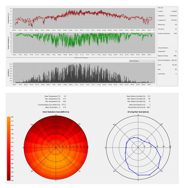
The direction with the most driving rain is south-southeast. There is a lot of solar radiation, with higher drying capacity than that towards most other orientations. Therefore, the southeast orientation is used for analyses of plastered walls, with still a lot of driving rain but slightly less drying capacity. For ventilated facades, straight north is always the decisive orientation.
