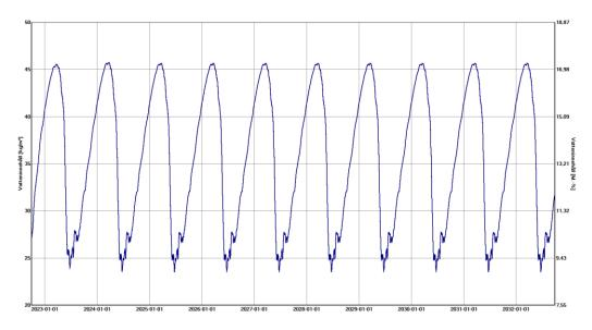
The wood fibreboard has the chance to dry out and the moisture content is always below the 18 M.-% which is considered the critical limit.
