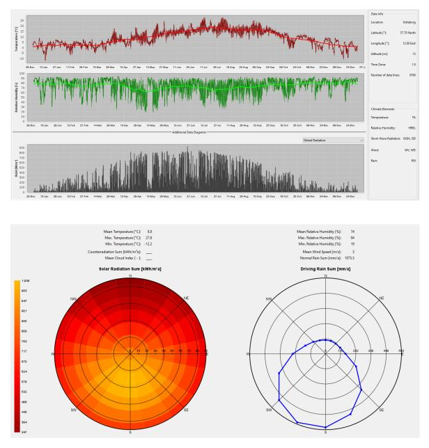
The direction with the most driving rain is south-southwest. There is a lot of solar radiation, with higher drying capacity than that towards most other orientations. Therefore, the southwest orientation is used for analyses of plastered walls, still with a lot of driving rain but slightly less drying capacity. For ventilated facades, straight north is always the decisive orientation.
