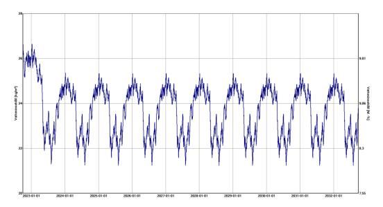
The wood fibreboard has the chance to dry out and the humidity is always below 10 M.-% and thus far below the critical limit.
