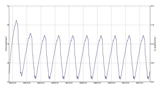
The wood fibreboard has the chance to dry out and the moisture content is always below 16 M.-% which is below the critical limit.
