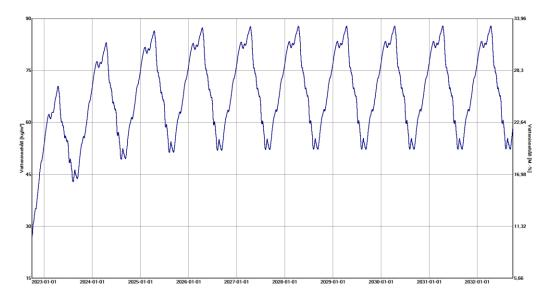
The wood fibreboard does not have the chance to dry out and the moisture content rises initially to stay all the time above the 18 M.-% which is considered the critical limit. Mould growth is likely and it is therefore not recommended to build in this way in the Bergen area.
