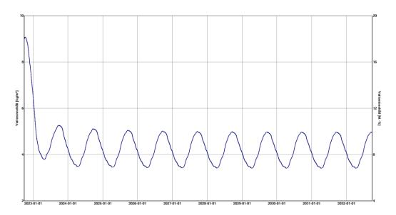
A low moisture level is reached after only a few months. Even with the intentionally high value at the beginning, the water content drops quickly and stays below 12 M.-%.
