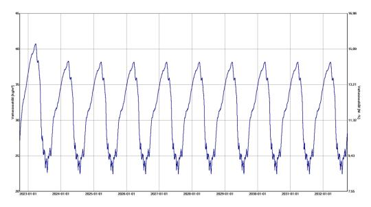
The wood fibreboard has the chance to dry out and the moisture content is always below 15 M.-% and thus below the critical limit.
