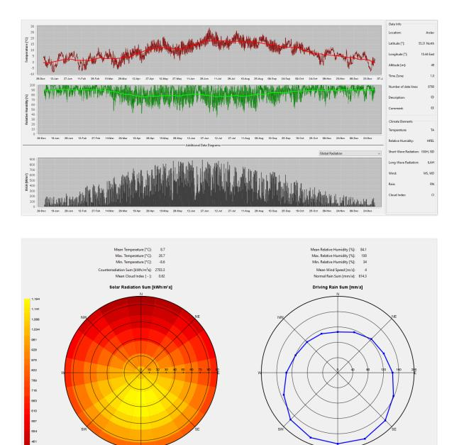
The direction with the most driving rain is south. There is also the strongest solar radiation, with high drying capacity. Therefore, the southeast orientation is used for analyses of plastered walls, with still high driving rain, but less drying from solar irradiation. For ventilated facades, straight north orientation is always the decisive one.
