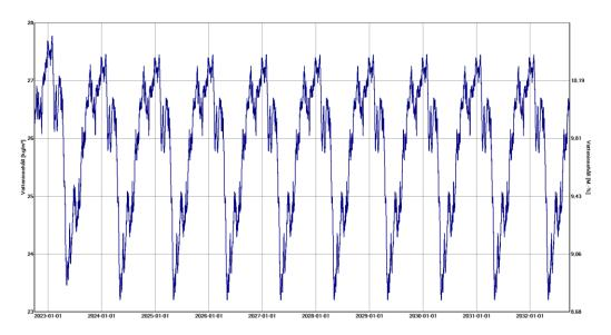
The wood fibreboard has the chance to dry out and the moisture content is always below 11 M.-% and thus far below the critical limit.
