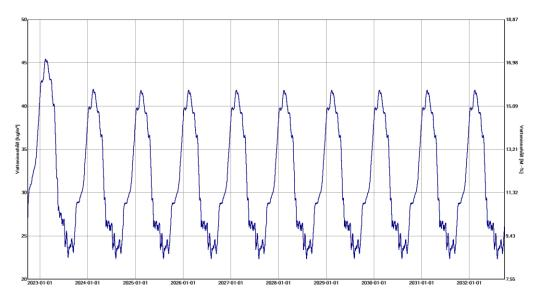
The wood fibreboard has the chance to dry out and the water content is always below 16 M.-% and thus below the lowest critical limit.
