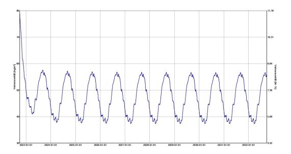
A low moisture level is reached after only a few months. Even with the intentionally high value at the beginning, the water content drops quickly and stays below 9 M.-%.
