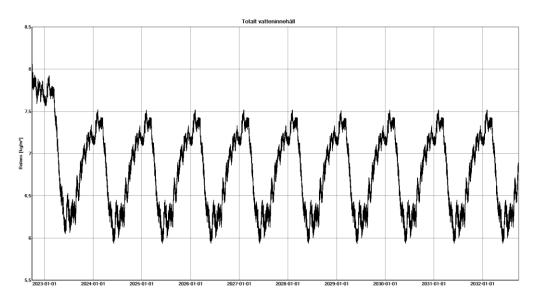
The simulation over 10 years shows that there is no accumulation of moisture over the long term and it takes only one season to release the assumed high level of built-in moisture. No risk of damage to the building fabric, or mould, can be expected if the work is carried out correctly.
