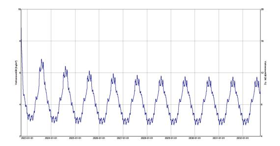
A low moisture level is reached after only a few months. Even with the intentionally high value at the beginning, the water content drops quickly and stays below 12 M.-%.
