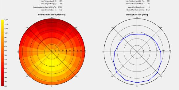
The direction with the most driving rain is straight south. There is also the strongest solar radiation, with high drying capacity. However, for the investigation on ventilated facades, straight north is always the decisive orientation.
