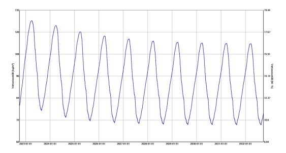
After a few seasons of stagnation, the water content is permanently below 17 M.-%. The use of dry materials at the time of construction will also eliminate the higher moisture content shown at the beginning of the simulation.
