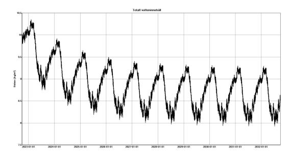
The simulation over 10 years shows that there is no accumulation of moisture over the long term, but it takes a few seasons to release the assumed high level of built-in moisture. No risk of damage to the building fabric, or mould, can be expected if the work is carried out correctly.
