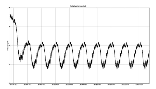
The simulation over 10 years shows that there is no accumulation of moisture over the long term and it takes only one season to release the assumed high level of built-in moisture. No risk of damage to the building fabric, or mould, can be expected if the work is carried out correctly.
