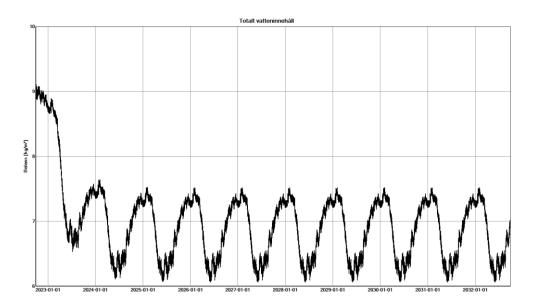
The simulation over 10 years shows that there is no accumulation of moisture over the long term, but it takes one season to release the assumed high level of built-in moisture. No risk of damage to the building fabric, or mould, can be expected if the work is carried out correctly.
