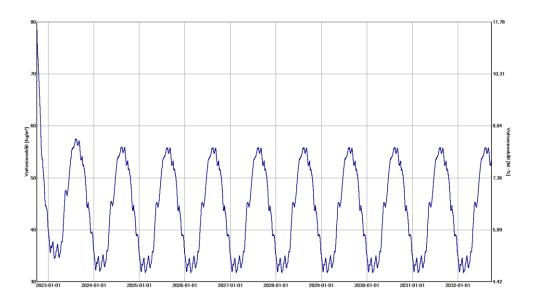
A low moisture level is reached after only a few months. Even with the intentionally high value at the beginning, the water content drops quickly and stays below 9 M.-%.
