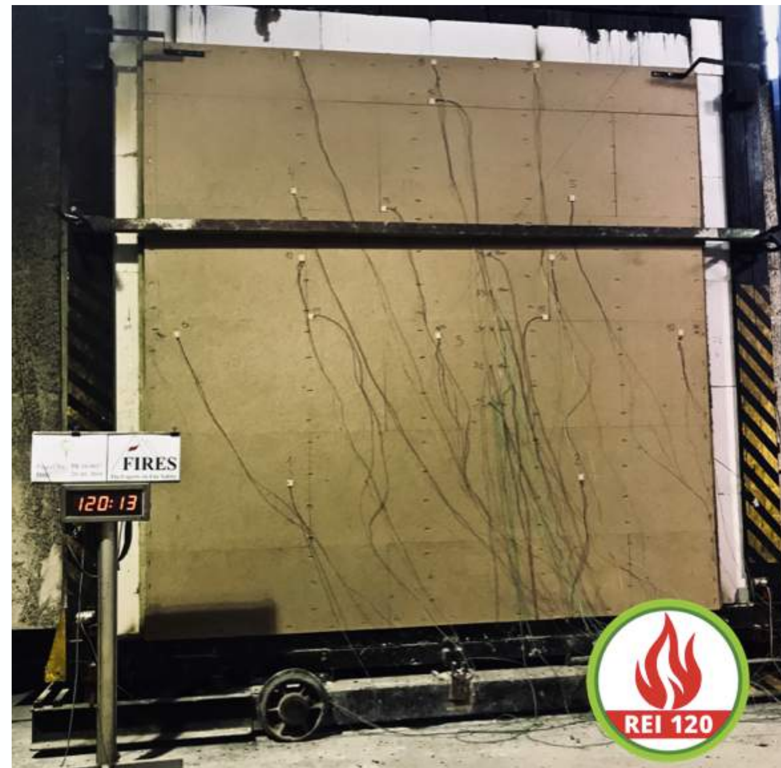
Fire test from interior
