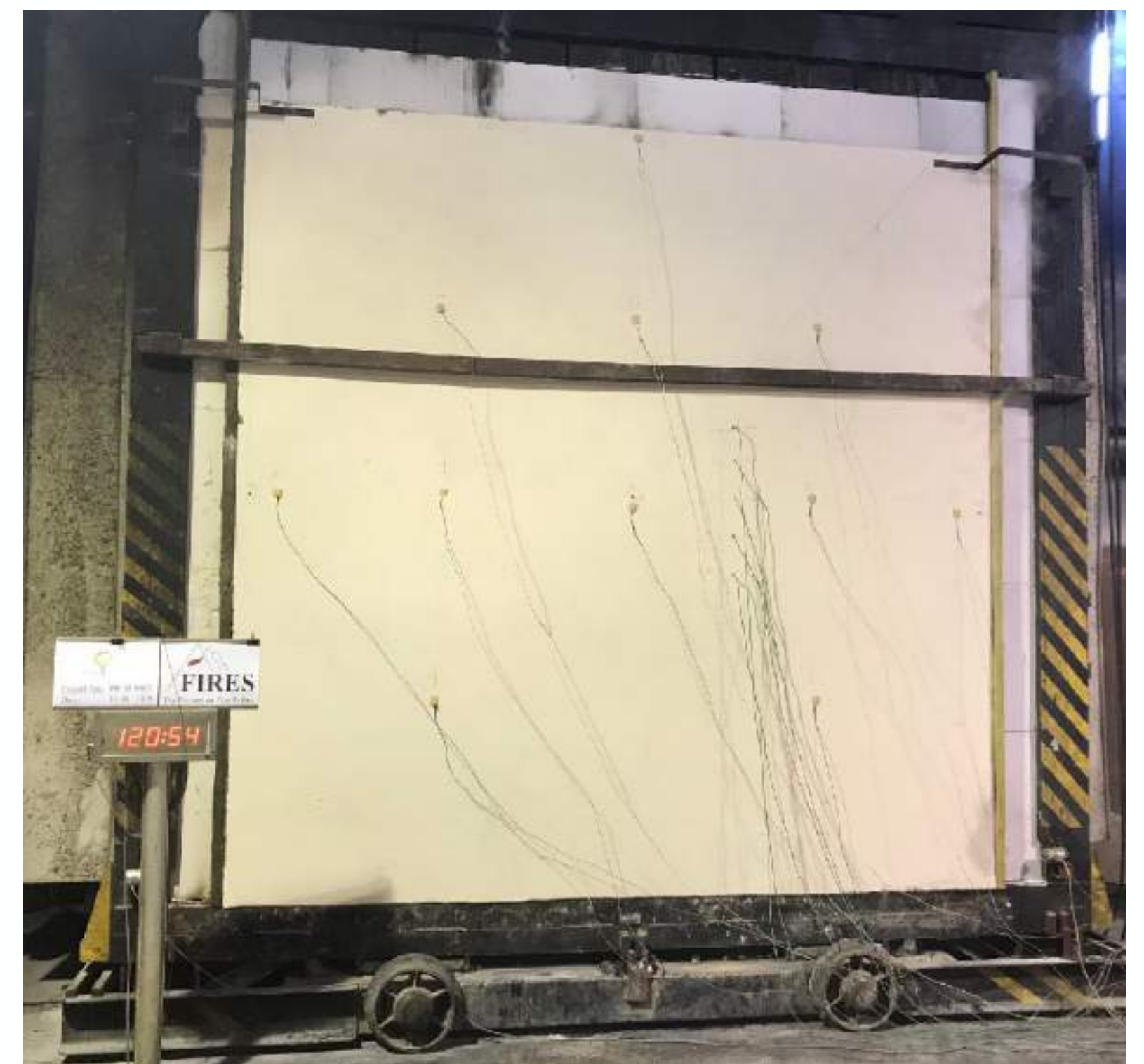
Fire test on exterior woodfibre layer Video 1min. 24 seconds
